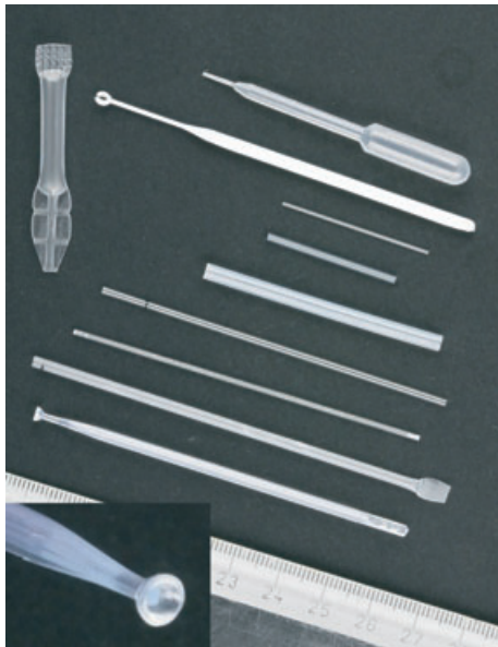
FIG 3. Transfer devices used to transfer capillary or venous blood to the RDT: pipettes (upper left and right), loop, capillaries, straws and inverted cup (below and insert). Some capillaries are very small, not easy to use and have no volume mark. The inverted cup proved to be the most accurate and safest blood transfer device [105].
