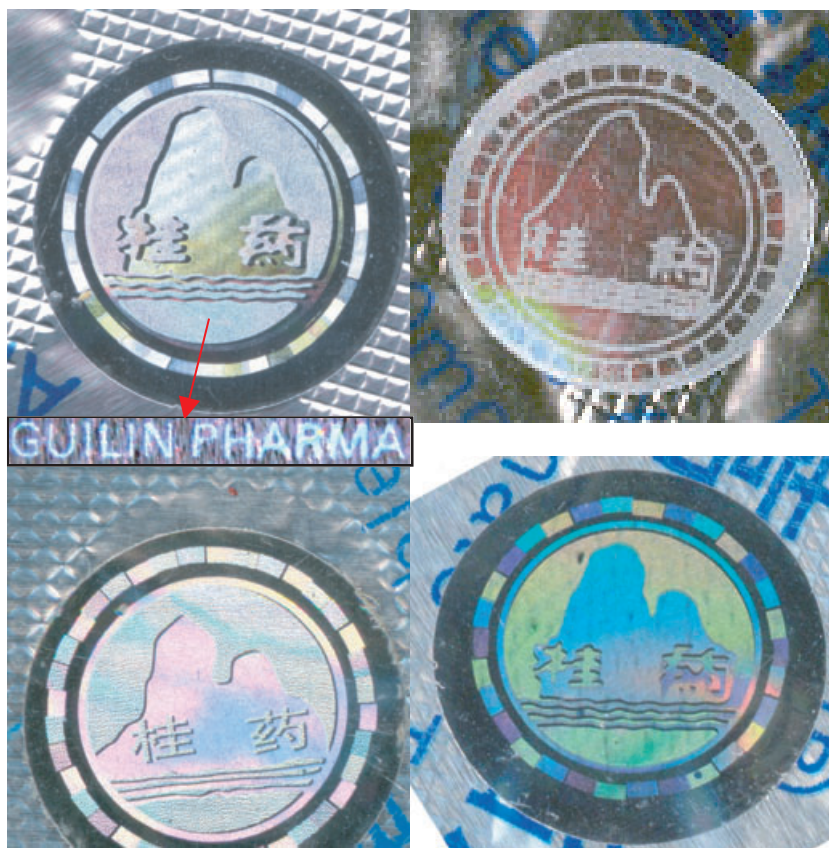
Figure 1 Evolution of counterfeited holograms on blisterpacks containing fake artesunate tablets. Top left, the genuine hologram. Top right, the first fake 'hologram', found after 1998, which lacked the three-dimensional appearance of a real hologram. Bottom left, the fake hologram, which started to appear in 2002–03 in Lao PDR and Cambodia, featuring a well-crafted hologram, but with a slightly different outline of the depicted mountains. Bottom right, the latest detected counterfeited hologram, almost indistinguishable from the genuine counterpart, but lacking the company name (only visible under magnification, arrow in top left picture).
