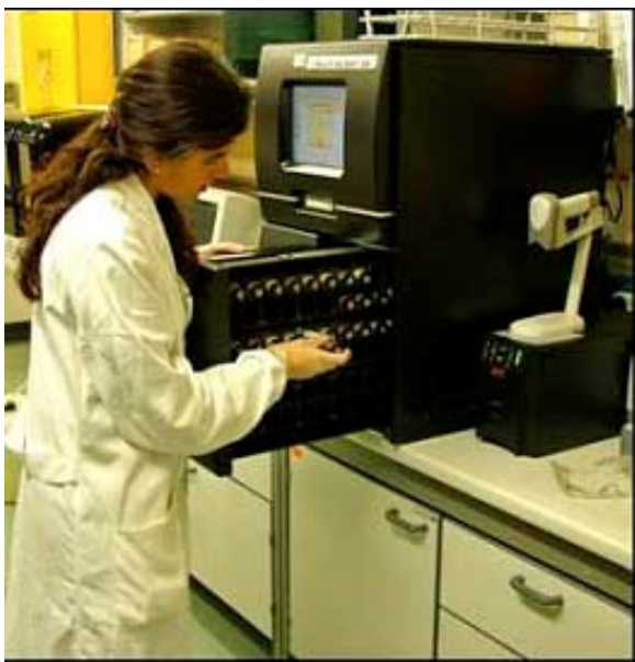
Figure 14-7: The BacT/Alert system
